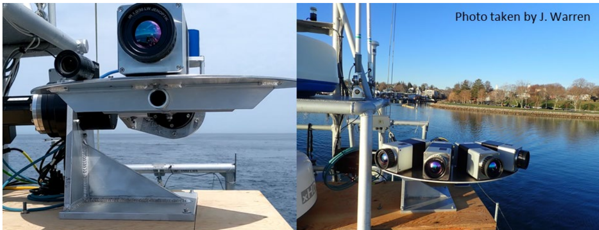
Figure 10. Refined version of the wide field of view thermal whale detection system using four cameras and providing a total of 120° field of view.
