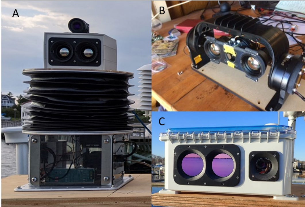
Figure 9. Evolution of the low-cost whale detection system: (A) version used in 2020 research cruises; (B) new miniaturized gimbal with two thermal cameras that can now be entirely mounted into an enclosure (C).
