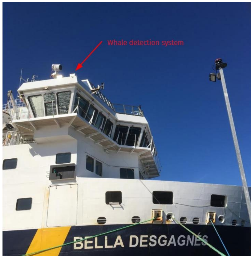
Figure 14: Whale detection system installed on M/V Bella Desgagnés .
