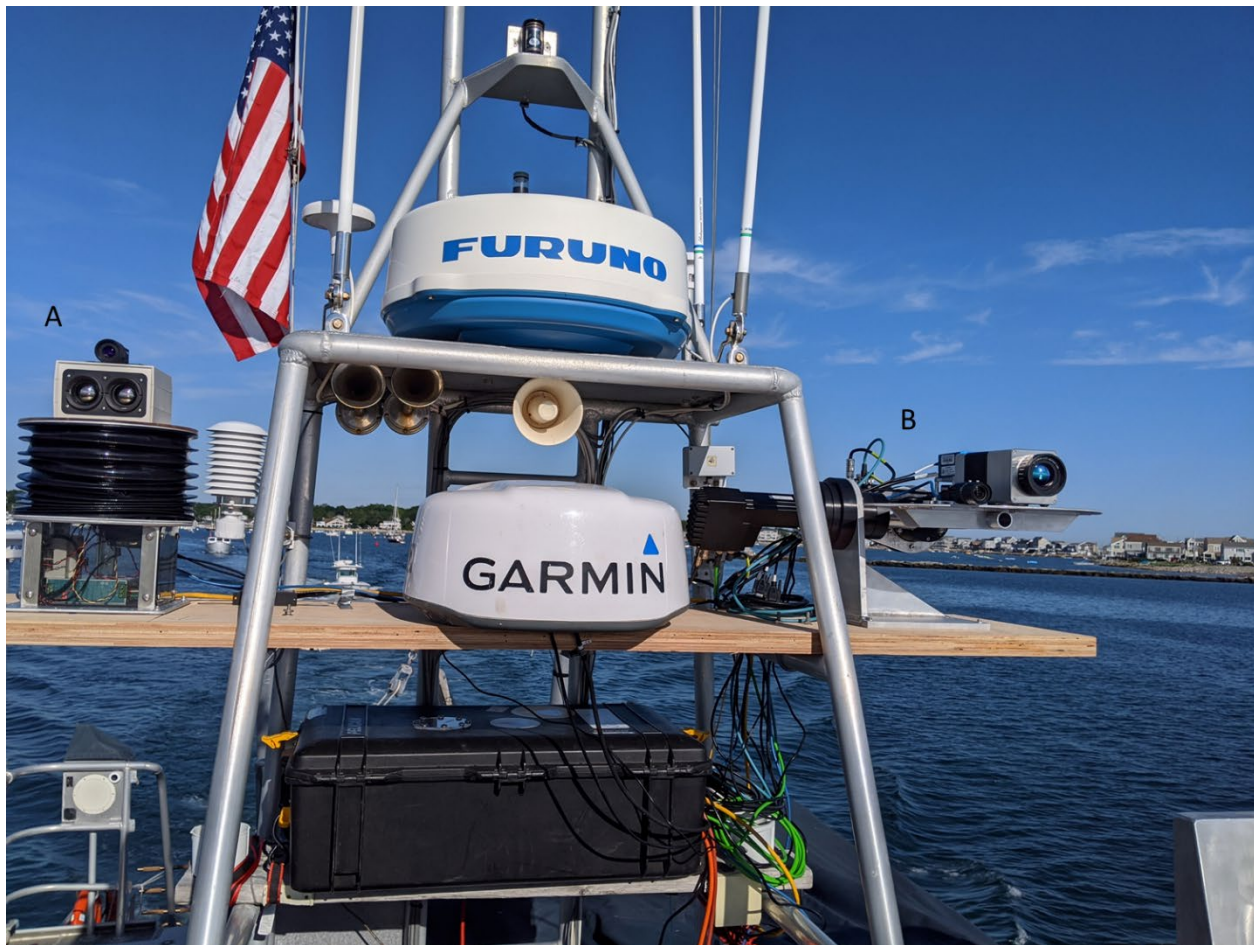
Figure 2. Installation of two thermal imaging-based whale detection systems on R/V Auk . (A) is a low-cost camera system for ship-strike mitigation; (B) is a higher-end system that allows for varying payload.
