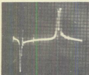
Fig. 8 - Actual Photograph of Voltage Pulse from Peaking Transformer
