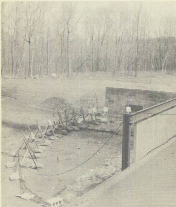
Figure 1 - Arc of Dipole Probes Used for Propagation and Incidental Modulation Studies
