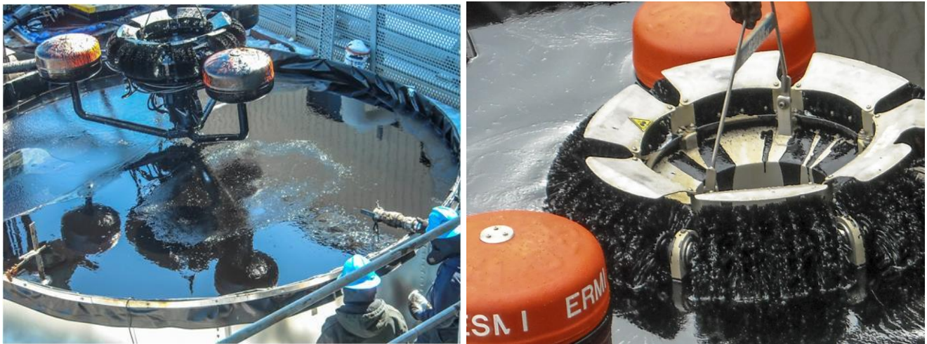
Figure 4. Helix skimmer during oil preload and testing.
