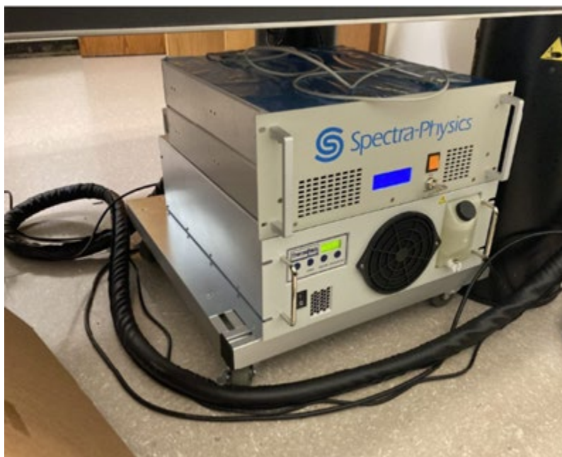
Figure 5. Installation – the power supply
