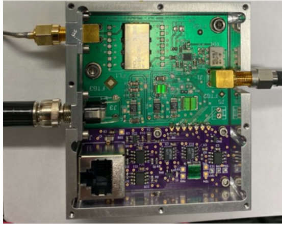
Figure 4: Ultra-low noise amplifier for trap radio-frequency (RF) potential. Left: picture of “Squaretron” with tailorable filtering and digital control of amplitude. Right: Comparison of phase noise frequency response for a standrad arbitray-waveform generator (AWG, Rigol DG1062Z ), a direct-digital synthesizer (Urukul, M-Labs), and the Squaretron.
