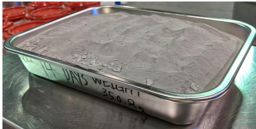
Figure 34: Displays the 316L powder after 14 days of humidification. The powder exhibited clumping and fusion in the upper exposed surface.
