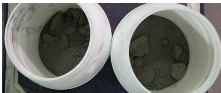
Figure 42: ALD-coated powders after humidification. 316L baseline coated in Al 2 O 3 amine terminated (left); 316L baseline coated in Al 2 O 3 (right).
