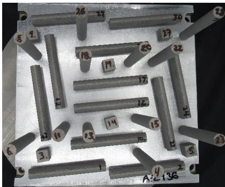
Figure 62: The printing layout for the A5083-RAM7 deliverable builds.
