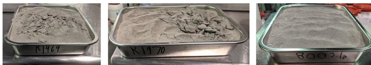
Figure 41: Stainless steel powder after 30-day humidification. 316L baseline coated in 7nm of Al 2 O 3 (left), 316L baseline coated in 7nm of Al 2 O 3 amine-terminated (middle), and 316L baseline (right).
