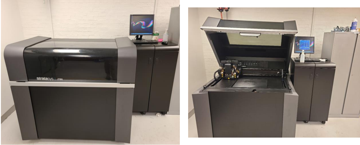
Figure 1. Stratasys J750 TM 3D printer installed at the University of South Carolina
