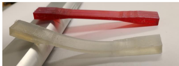
Figure 3. Vero stiff material in red and Tango compliant material in white
