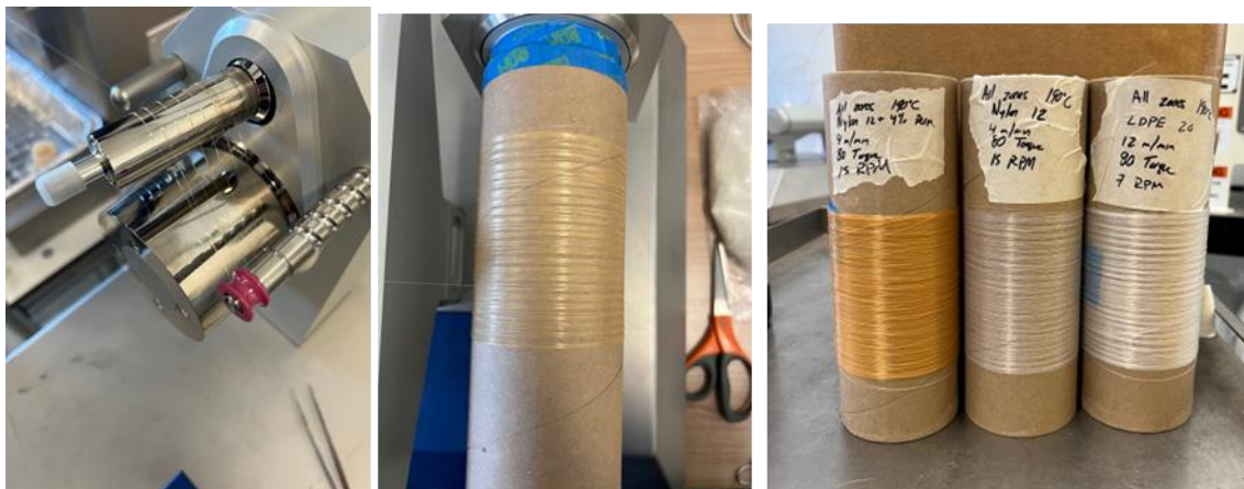
Figure 22. Demonstration of melt extrusion (left), collection onto a spool (center), and spools of composite filaments composed of permethrin-nylon-12, nylon-12, and LDPE (right).
