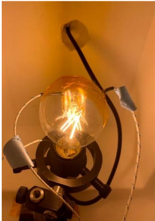
Figure 5. A19-TES Operation during testing with locations of the 3 thermocouples on adhered to the lamp with polyimide. A fourth thermocouple is adhered to the wall of the thermal chamber.
