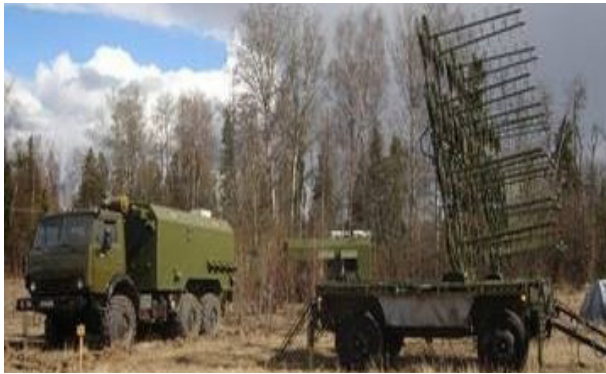
Deployed SATCOM jammer in the field. 445
