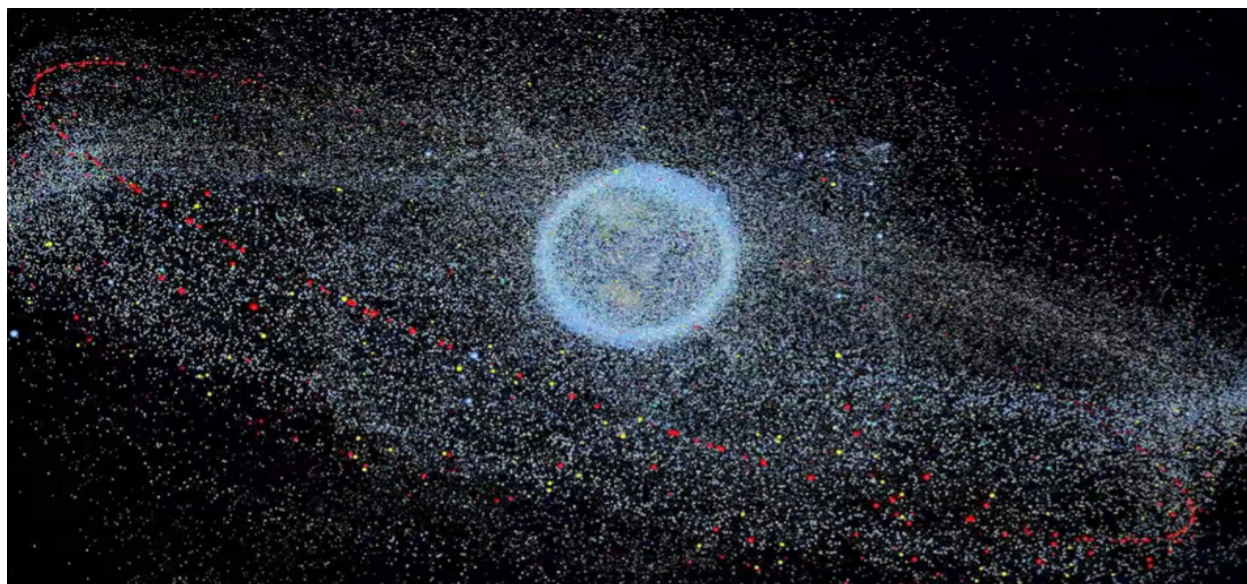
Computer rendering of tracked objects greater than 10 centimeters in Earth's orbit. Red, yellow, and green objects are representations of active satellites in the GEO orbital belt and in MEO. [Note: The objects are not drawn to scale; the objects are approximately 10,000 times greater than actual size.]
