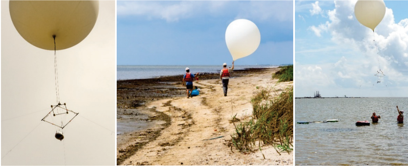
Figure 8. Photos of modified Picavet system ( left ); shoreline and mudflat ( middle ); balloon deployment ( right ). (Photos by Justin Wilkens.)
