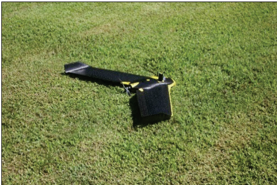
Figure 2. SenseFly eBeeRTK fixed-wing drone used to acquire aerial images. (Photo by Justin Wilkens.)
