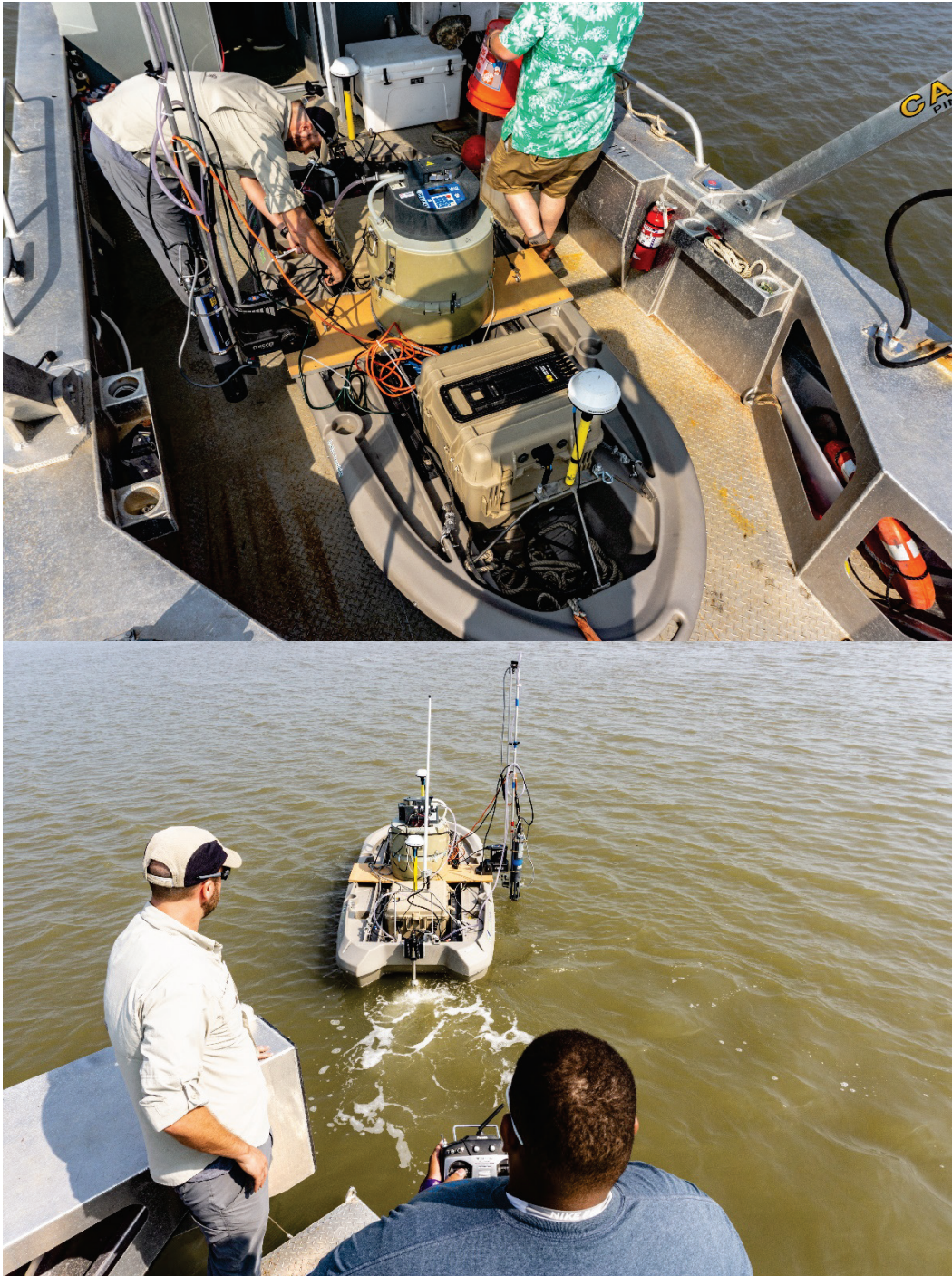
Figure 18. MARV transported to demonstration area in landing craft ( top image ). MARV measuring water quality as bulk carrier ship transits north in Calcasieu Ship Channel ( bottom image ). (Photos by Justin Wilkens.)
