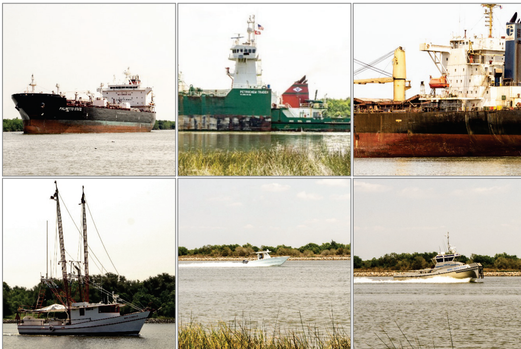
Figure 20. Example vessels monitored during the demonstration. Top row ( left to right ): oil/chemical tanker, pusher tug tanker, bulk carrier cargo. Bottom row ( left to right ): fishing, recreational, and fast response vessels. (Photos by Justin Wilkens.)
