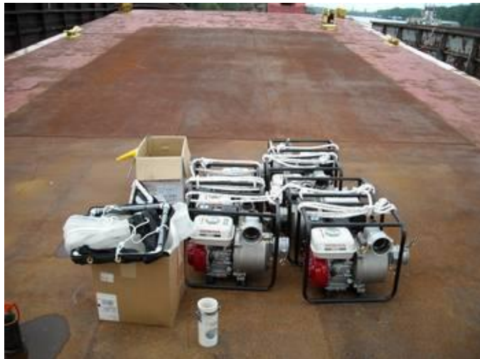
Pumps for emptying tanks
