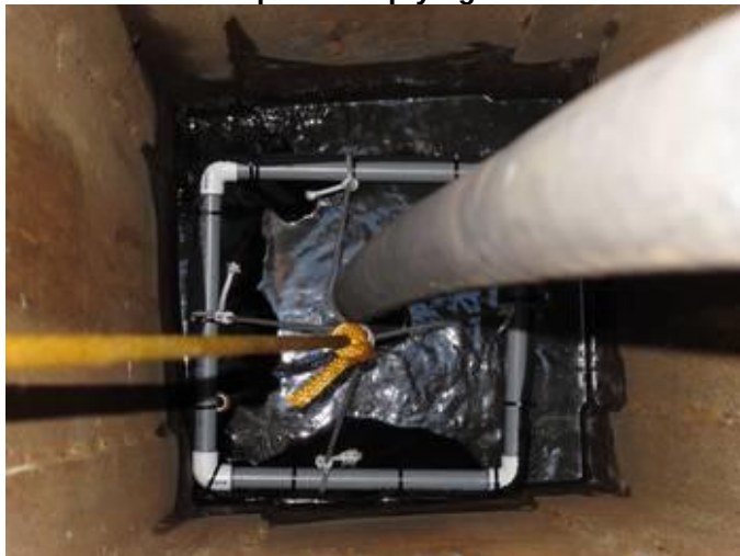
Emptying tank into plankton net in spud well
