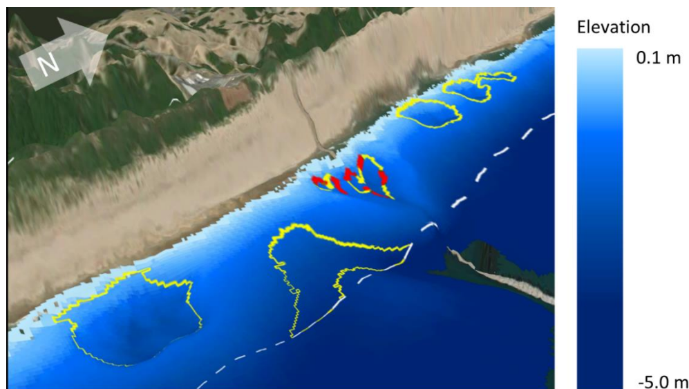
Fig. 3—A 3-D extruded graphic of part of the DEM for 2019-06-19. Satellite imagery has been draped over elevations above the 0-m contour. The increasingly saturated blue pixels are DEM elevations in the near shore (see color bar at right). Bathymetric depressions identified by de-trending are outlined in yellow. Two bathymetric depressions at the center (marked with a red-and-yellow dash) also meet the definition of a rip channels. The dashed, white line shows the seaward boundary of the area analyzed, a 150-m buffer from the shoreline.
