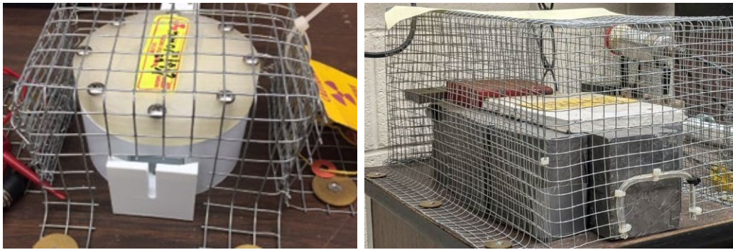
Fig. 8 RIs (left) ^{63}\text{Ni} and (right) ^{147}\text{Pm} are housed in pillboxes that include a drawer to insert the EC cartridges
