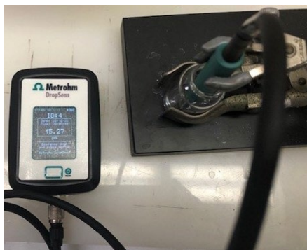
Figure 3.2.18. Electrochemical reader (Metrohm) connected to BDD SPE electrode immersed in solution of 20 v % CH 3 CN+Britton-Robinson buffer at pH 2 in the presence of 42 ppm 2-CEES. The reader shows 15.7 ppm 2-CEES.
