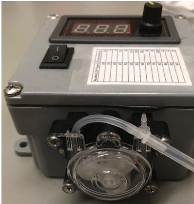
Figure 4.10. Pump, motor controller and a 12V battery packaged together
