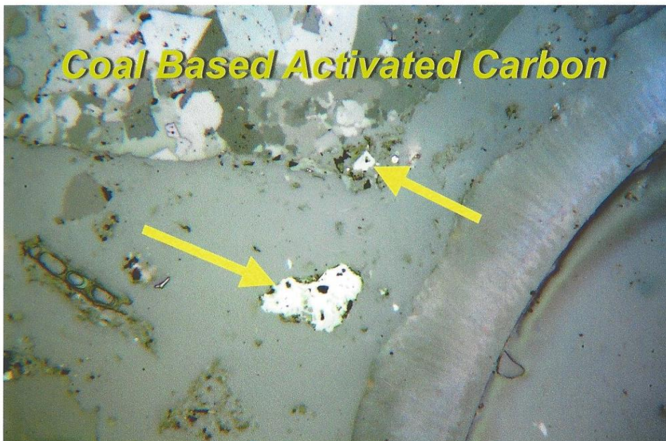
Figure 9: Photomicrographs of Koppers Samples 2020-0714 thru 2020-0720 from Geosyntec (Sediment 9- 0510, 1015 & 1520, 7-DUP-1015, 1520, 0510 & 0005) Showing; Seashell, Fine Sized Groundmass Materials, Coal Based Activated Carbon and Metallic Inclusions in Coarse Rock. Reflected Polarized Light In Air, X250.
