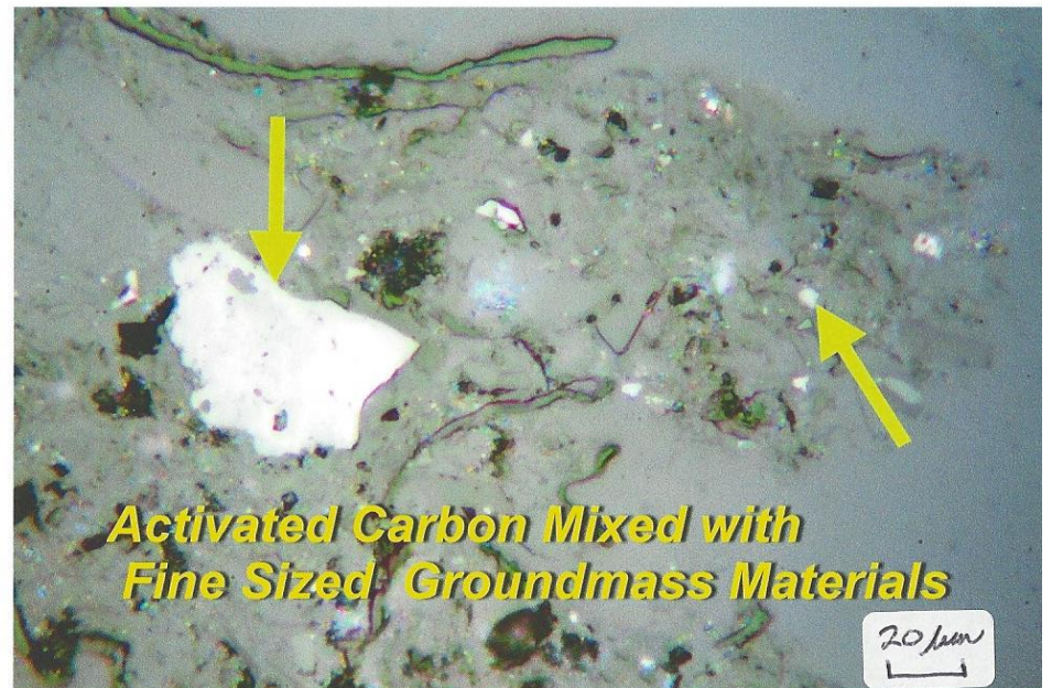
Figure 12: Photomicrographs of Koppers Samples 2020-0714 thru 2020-0720 from Geosyntec (Sediment 9- 0510, 1015 & 1520, 7-DUP-1015, 1520, 0510 & 0005) Showing; Coarse Quartz-like Mineral, Fine Size Groundmass Mineral Matter, Plant Material – organic and Activated Carbon. Reflected Polarized Light In Air, X600.
