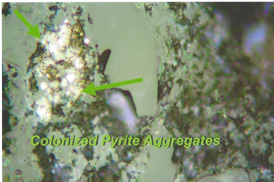
Figure 13: Photomicrographs of Koppers Samples 2020-0701 thru 2020-0707 from Geosyntec (Sediment 4-1520, 0510, 0005 & 1015, 5-0510, 1520 & 1015) Showing; Calcite, Other Coarse MM, Partially Soluble MM, Pyrite Aggregate and Activated Carbon Mixed with Groundmass Mineral Matter. Reflected Light In Air, X600.
