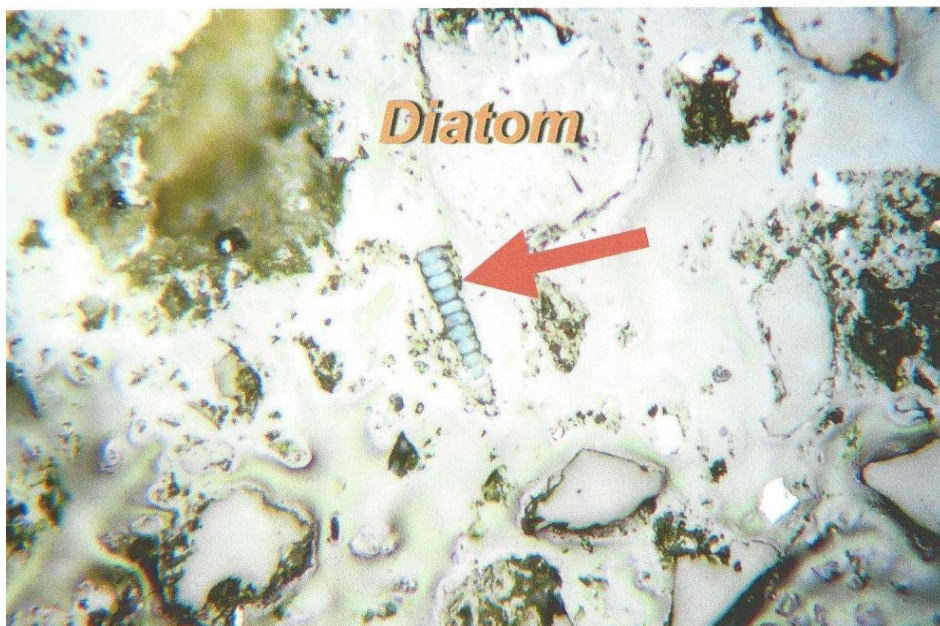
Figure 8: Photomicrographs of Koppers Samples 2020-0708 thru 2020-0713 from Geosyntec (Sediment 6-1520, 0510 & 0005, 7-1520, 0005 & 0510) Showing; Fine Grain Plant Material, Charcoal Structure, Diatom and Seashell – Carbonate. Reflected Polarized Light In Air, X250.
