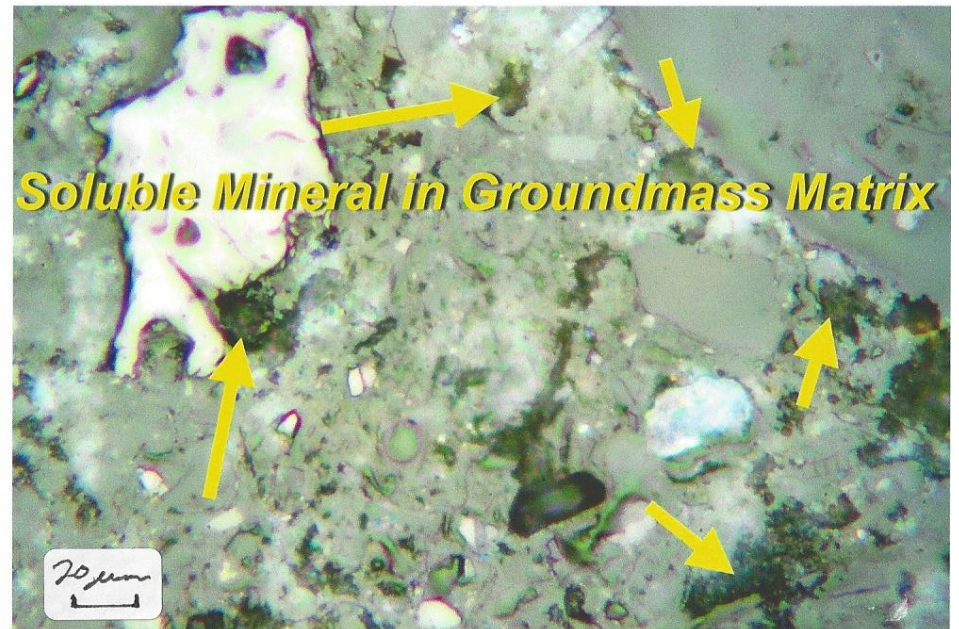
Figure 13: Photomicrographs of Koppers Sample 2020-0081 thru 20-0086 of Sediment Samples from Geosyntec (T82-2, 3, 5, 6, 7 & 9) Showing; Plant Material in Groundmass Matrix, Quartz, Activated Carbon, Pyrite in Groundmass Matrix and Soluble Mineral in Groundmass. Reflected Light In Air, X600.
