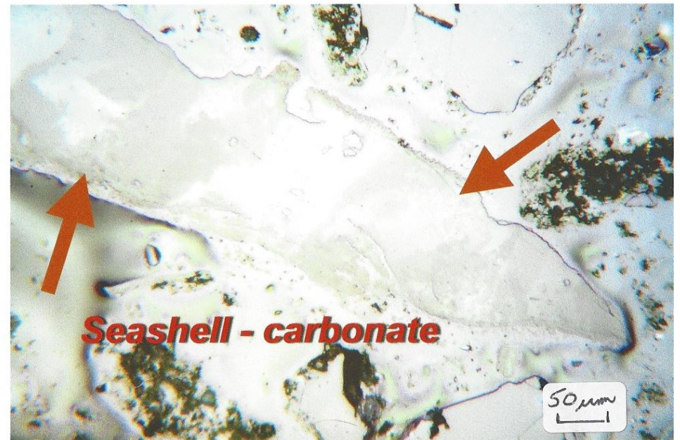
Figure 8: Photomicrographs of Koppers Samples 2020-0708 thru 2020-0713 from Geosyntec (Sediment 6-1520, 0510 & 0005, 7-1520, 0005 & 0510) Showing; Fine Grain Plant Material, Charcoal Structure, Diatom and Seashell – Carbonate. Reflected Polarized Light In Air, X250.
