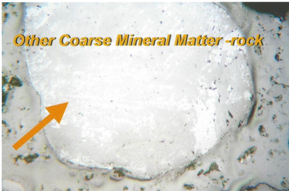
Figure 7: Photomicrographs of Koppers Samples 2020-0708 thru 2020-0713 from Geosyntec (Sediment 6-1520, 0510 & 0005, 7-1520, 0005 & 0510) Showing; Coarse Carbonate (limestone), Quartz Like Coarse Mineral Matter, Other Coarse Mineral Matter (rock) and Activated Carbon. Reflected Light In Air, X250.
