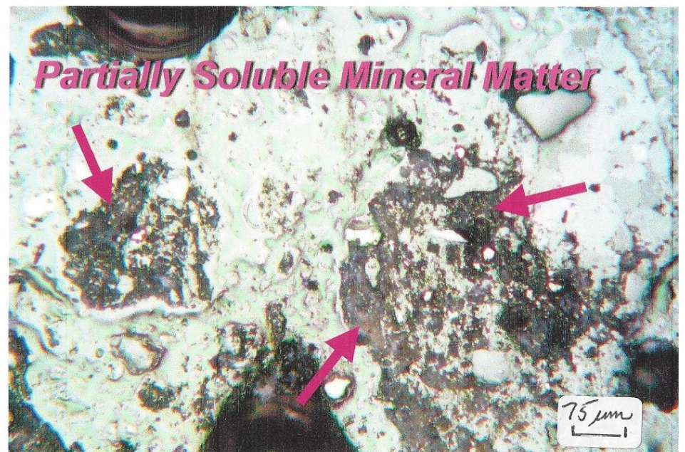
Figure 8.) Photomicrographs of Koppers Samples 2020-0695 thru 2020-0700 from Geosyntec (Sediment 2-1520, 0005 & 1015, 3-0510,1520 & 1015) Showing; Plant Material – organic, Activated Carbon -Coal Based, Groundmass MM and Partially Soluble Mineral Matter. Reflected Polarized Light In Air, X135.
