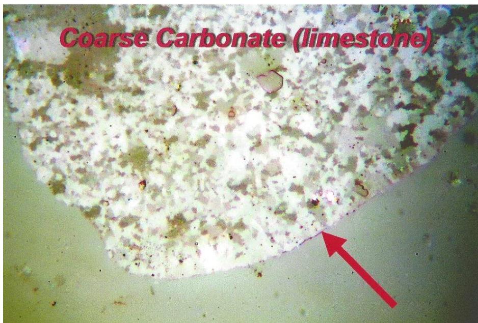
Figure 10.) Photomicrographs of Koppers Samples 2020-0695 thru 2020-0700 from Geosyntec (Sediment 2-1520, 0005 & 1015, 3-0510, 1520 & 1015) Showing; Plant Material, Activated Carbon (coal based), Coarse Carbonate (limestone) and Partially Soluble Groundmass Mineral Matter. Reflected Polarized Light In Air, X600.
