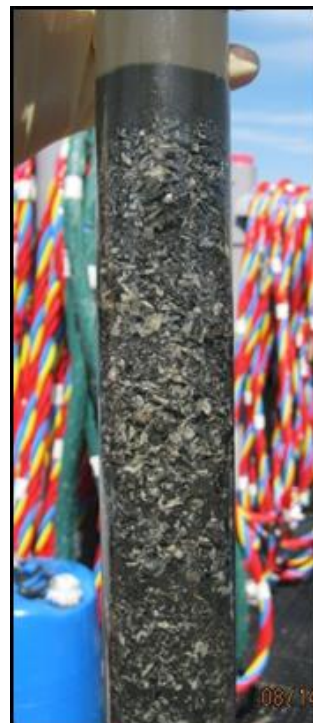
Figure 13. Sediment core from Pier 7 for sectioning and analysis.
