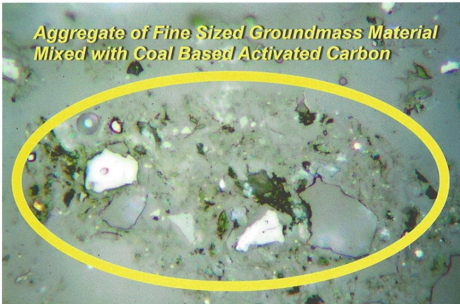
Figure 12: Photomicrographs of Koppers Samples 2020-0708 thru 2020-0713 from Geosyntec (Sediment 6-1520, 0510 & 0005, 7-1520, 0005 & 0510) Showing; Activated Carbon Mixed with Groundmass MM, Pyrite in Coarse MM, Aggregate of Fine Sized Groundmass and Coal Based Activated Carbon. Reflected Light In Air, X600.
