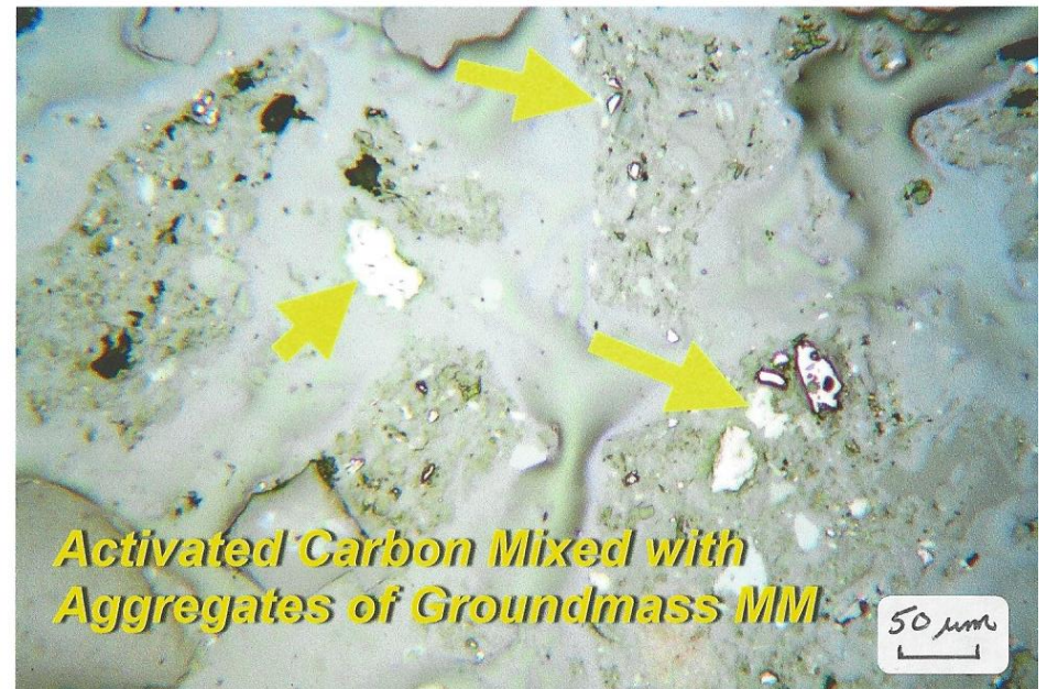
Figure 7: Photomicrographs of Koppers Samples 2020-0708 thru 2020-0713 from Geosyntec (Sediment 6-1520, 0510 & 0005, 7-1520, 0005 & 0510) Showing; Coarse Carbonate (limestone), Quartz Like Coarse Mineral Matter, Other Coarse Mineral Matter (rock) and Activated Carbon. Reflected Light In Air, X250.
