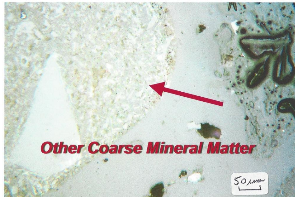
Figure 8: Photomicrographs of Koppers Samples 2020-0714 thru 2020-0720 from Geosyntec (Sediment 9- 0510, 1015 & 1520, 7-DUP-1015, 1520, 0510 & 0005) Showing; Carbonate – Seashell, Carbonate – limestone-like, Quartz-like Mineral and Other Coarse Mineral Matter. Reflected Polarized Light In Air, X250.
