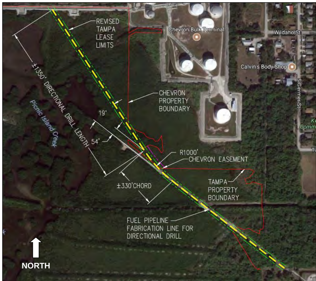
Figure 2-5. Aerial of Replacement Using Horizontal Directional Drill
