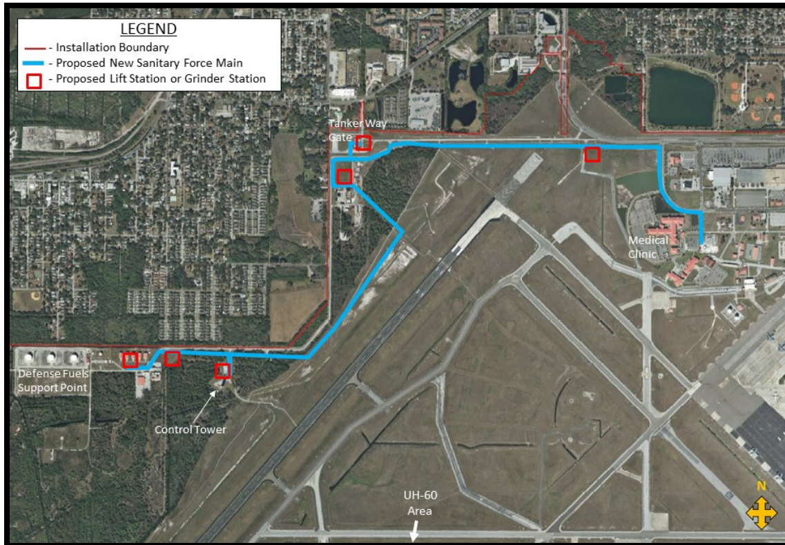
Figure 2.2: General route for expanding the sanitary sewer along the Northern Route Alternative.
