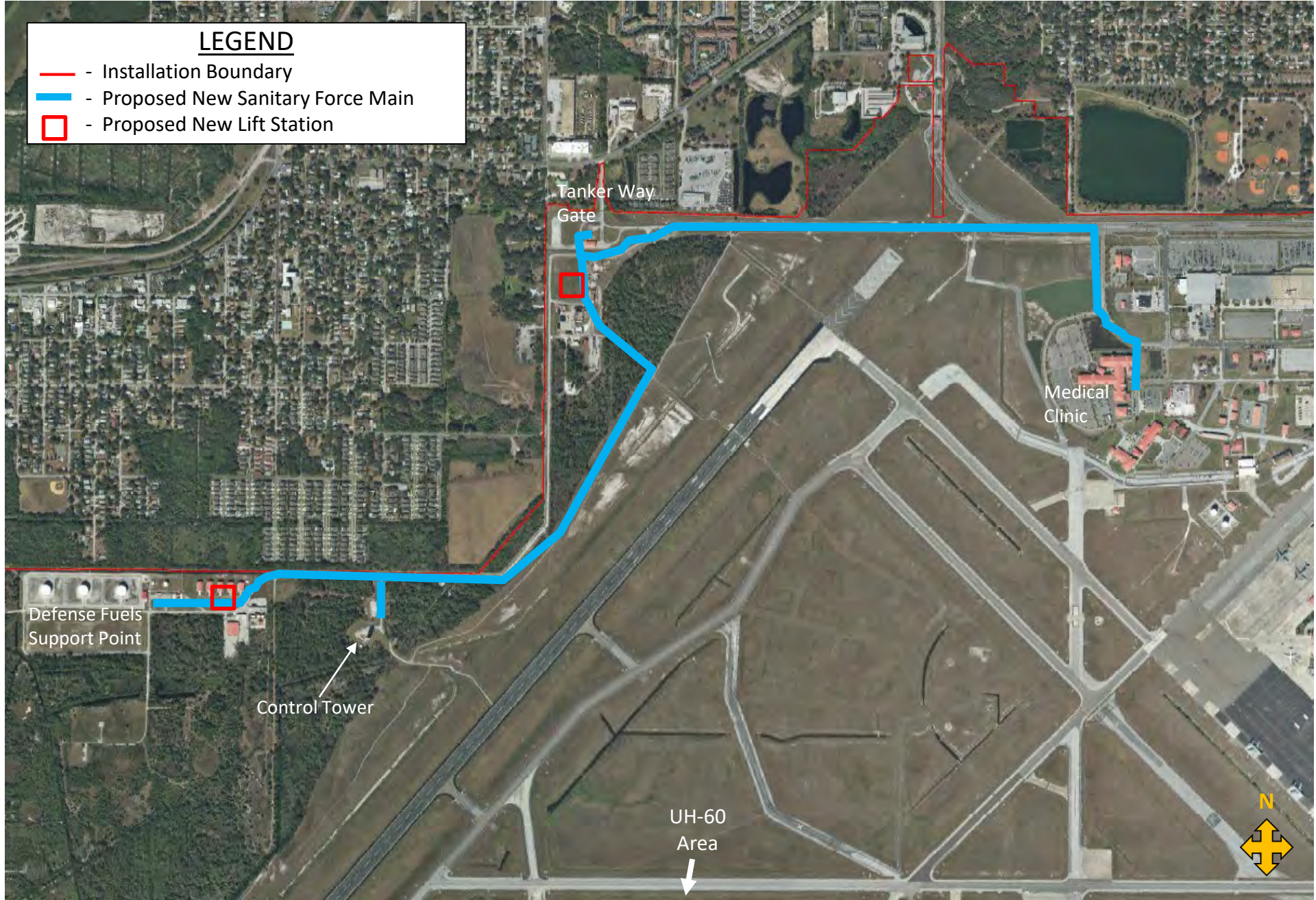
Figure 2: Location of proposed force main piping for the Northern Route Alternative considered for expansion of the sanitary sewer system to the western side of the installation.
