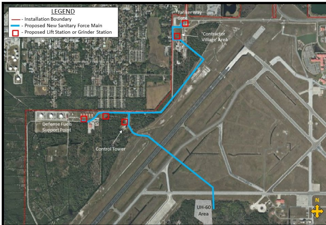
Figure 2.1: General route identified for expansion of sanitary sewer system under the Preferred Alternative.
