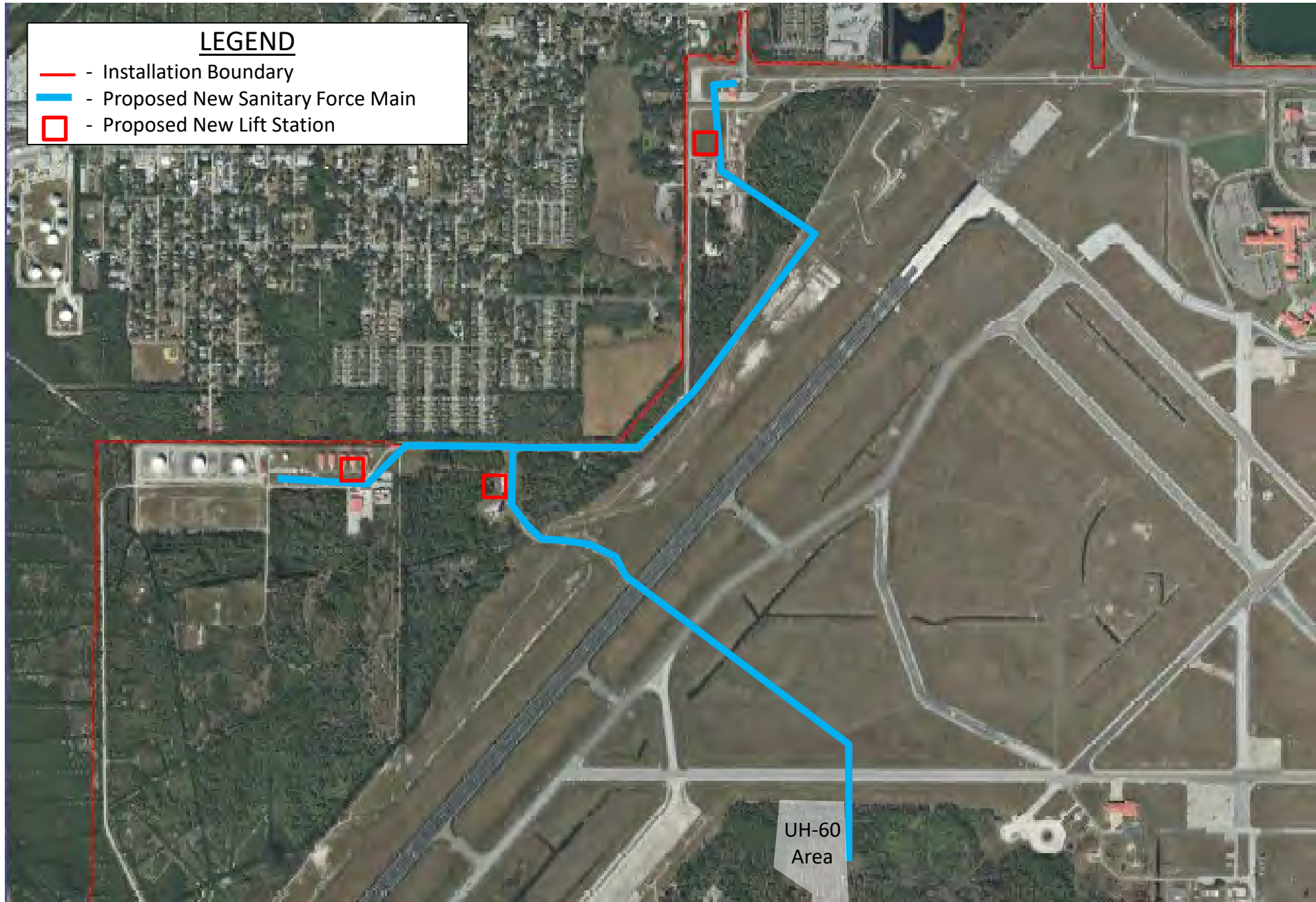
Figure 1: Location of the proposed force mains to support expansion of the sanitary sewer system to the western side of the installation.
