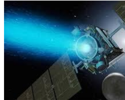
DAWN (Xenon Ion Engine) ~11 km/s Delta-V
