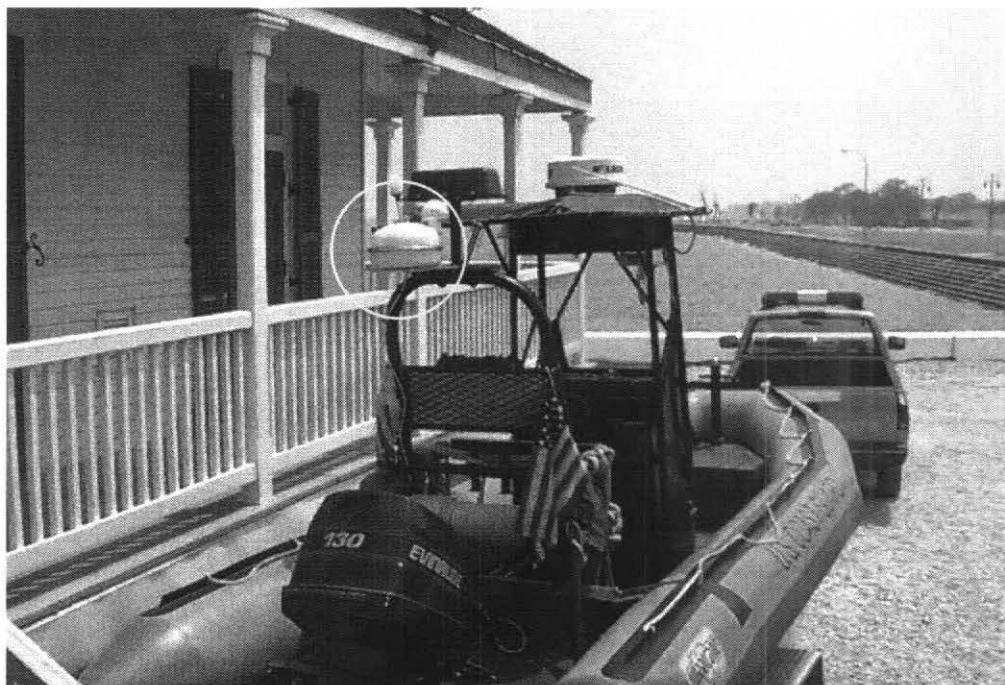
Figure 3-12. 19 FT RHIB looking forward from stern. Note the BOATRACS antenna mounted on a plate behind the Blue Light (outlined in white).
