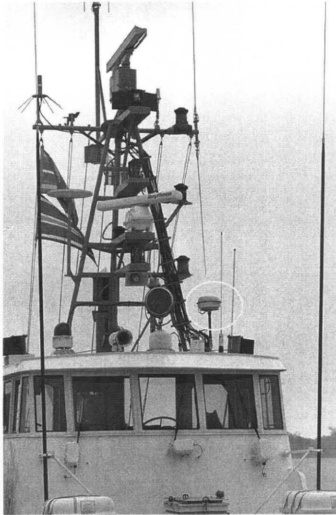
Figure 3-5. USCGC POINT WINSLOW, standing on bow looking aft. BOATRACS Antenna is mounted on a standoff on the Port side of the Pilot House roof (outlined in white)
