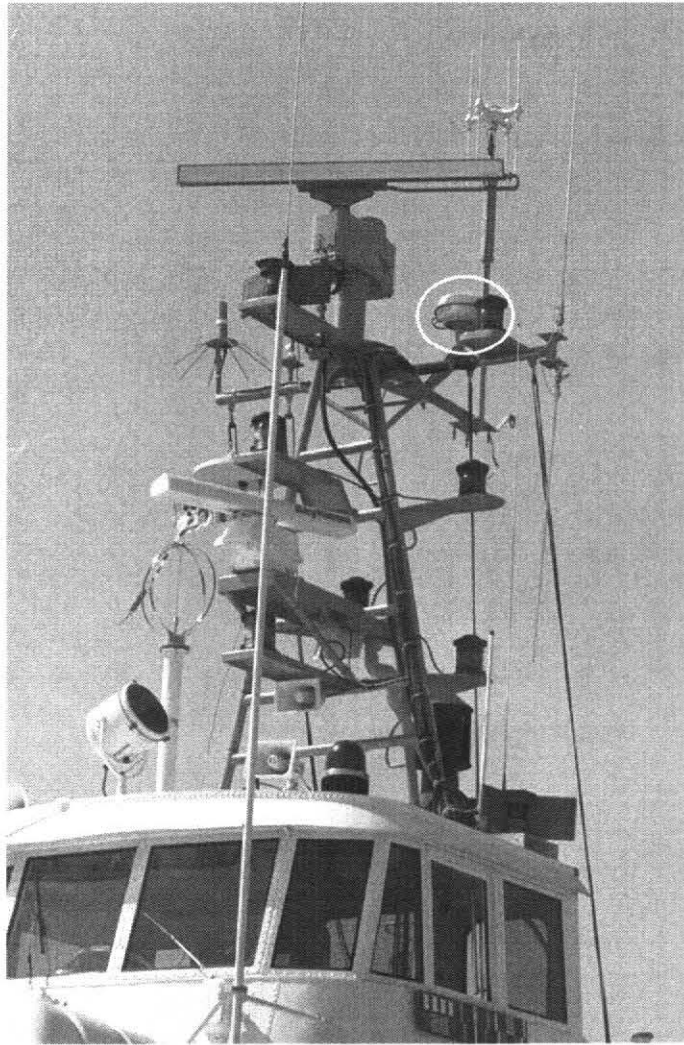
Figure 3-3. USCGC POINT SAL, standing on dock looking at Port side and mast. Note the BOATRACS antenna (small dome) mounted below and to the right of the RADAR antenna (outlined in white).
