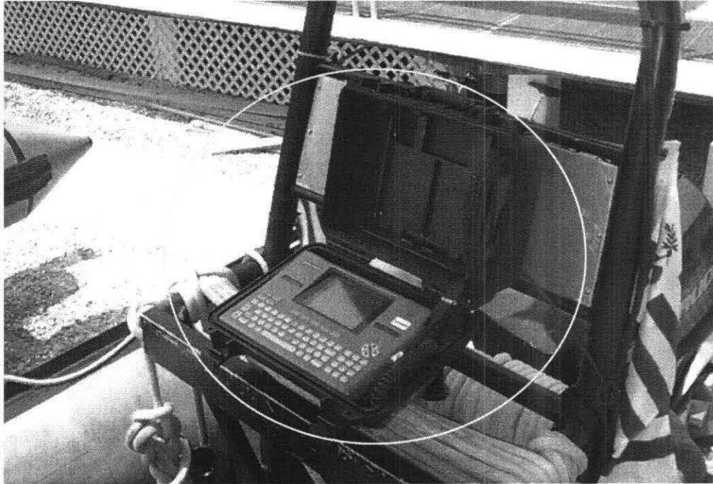
Figure 3-13. 19 FT RHIB, looking aft from cox'n's station. Note the BOATRACS Enhanced KDU mounted inside of a Pelican case on the front side of the rollbar.
