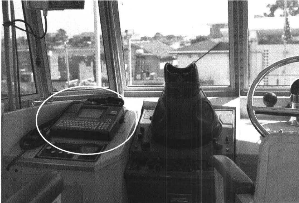
Figure 3-4. 3 POINT SAL, inside of pilothouse looking forward. Note the BOATRACS Enhanced Keyboard Display Unit mounted on the console to the left of the RADAR screen (outlined in white).
