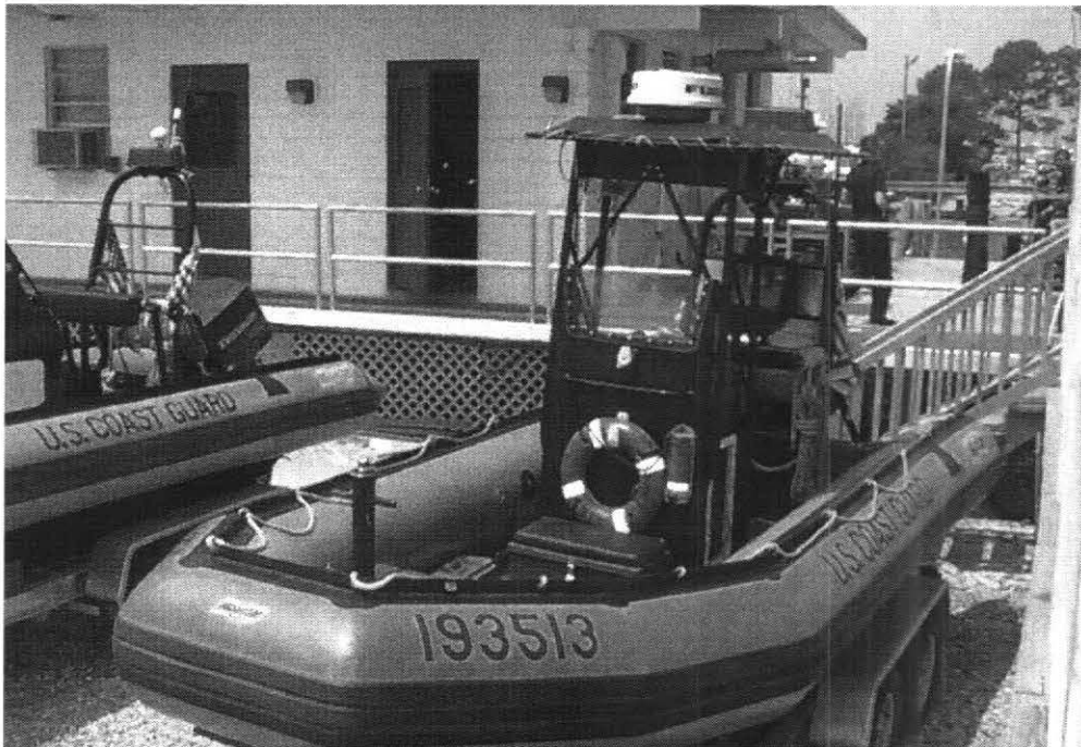
Figure 3-11. 19 FT RHIB, CG 193513, USCG Station New Orleans, LA. This boat is trailered to the desired location and then put into the water.
