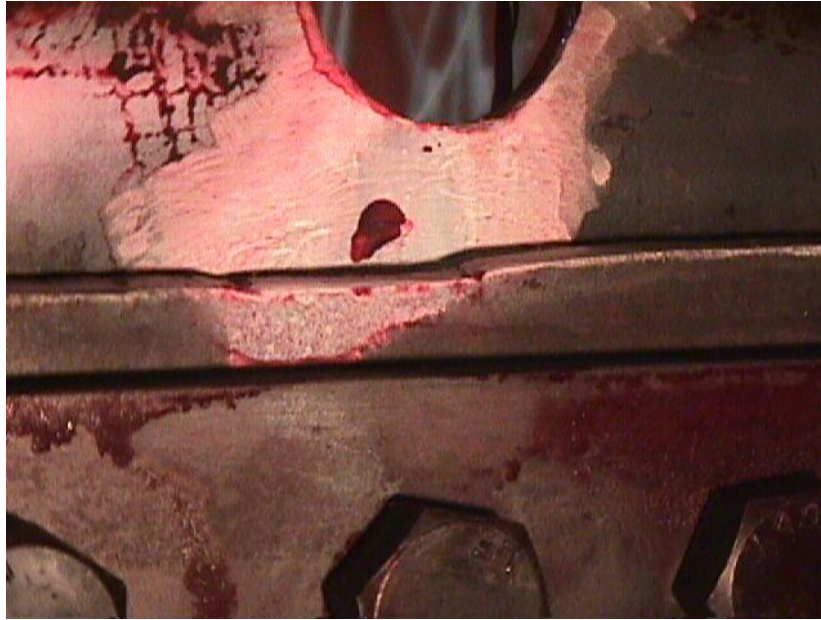
Figure 11-21: Re-initiation of crack from internal weld defect.
