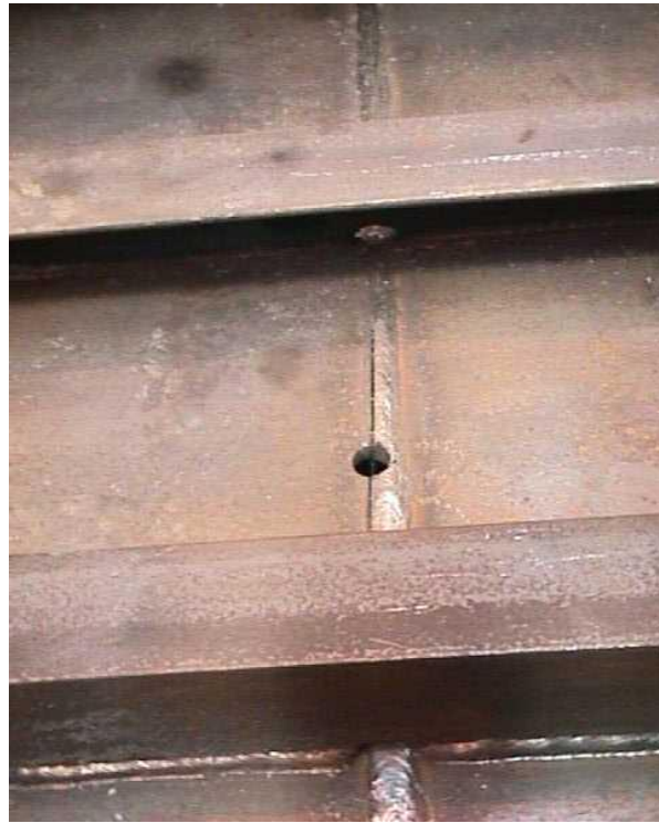
Figure 3-14: Typical initial crack introduced in specimen with reciprocating saw.
