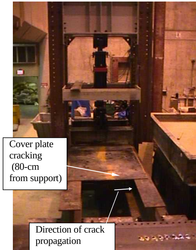
Figure 11-26: Cover plate detail prior to repair with and crack propagation direction indicated.
