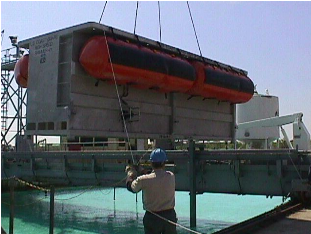
Figure 2. JBF Skimmer being lowered into test tank.
