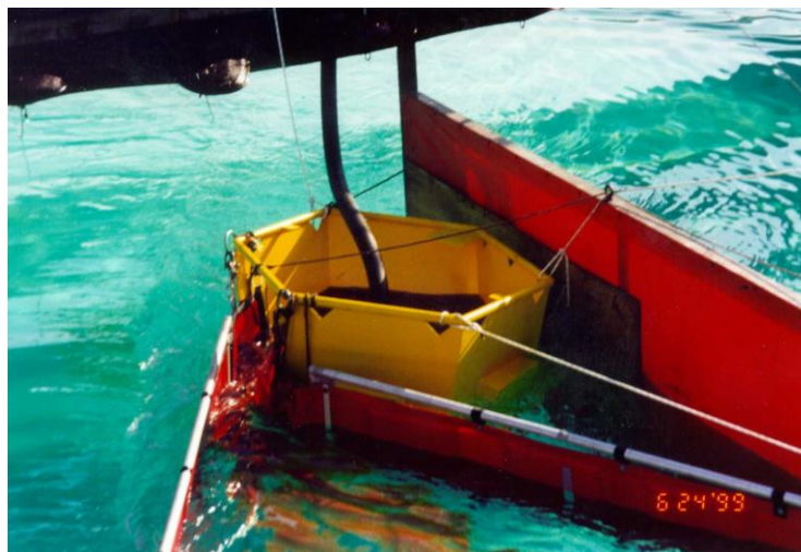
Figure 21. Circus Skimmer with Sweeping Arms Positioned 12” from the Top of Hull.
