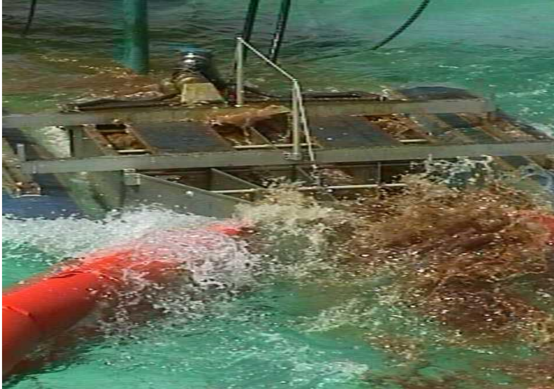
Figure 17. FasFlo Skimmer in Harbor Chop Waves.
