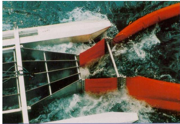
Figure 13. Expansion Zone to produce Laminar Flow.
