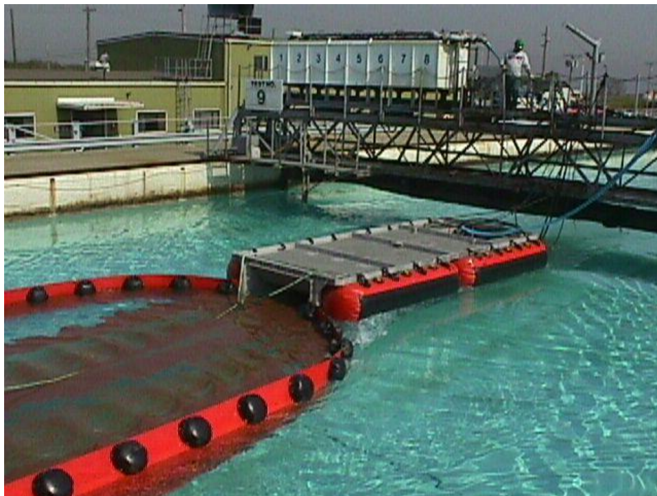
Figure 4. JBF Skimmer Test Setup with Applied Fabrics Globe Boom.
