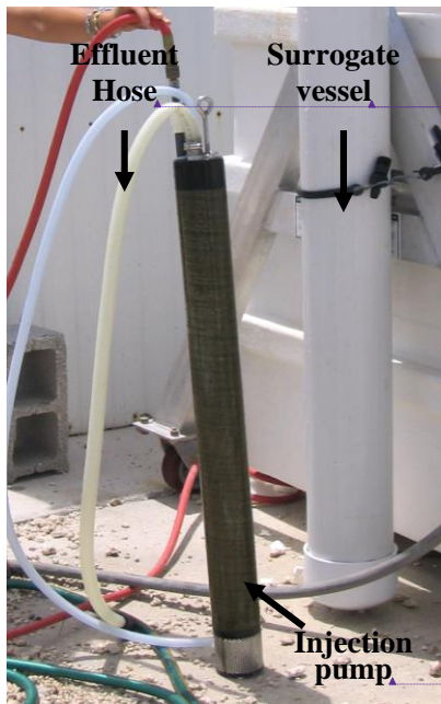
Figure 7. Surrogate injection: Auto-reclaimer pump (left-hand side) with adjacent surrogate vessel (right-hand side). Pump is placed inside the vessel containing surrogates where it pumps the surrogates up through the pump and out the hose at the top.
