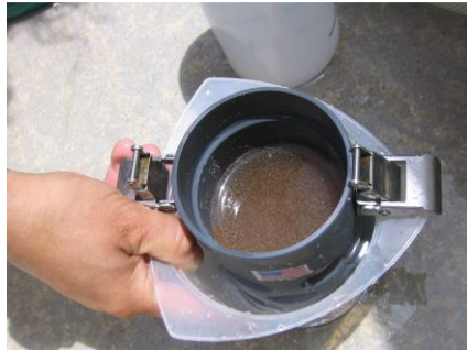
Figure 11. Collection and concentration of injected surrogate ( Artemia ) in the detachable cod-end.
