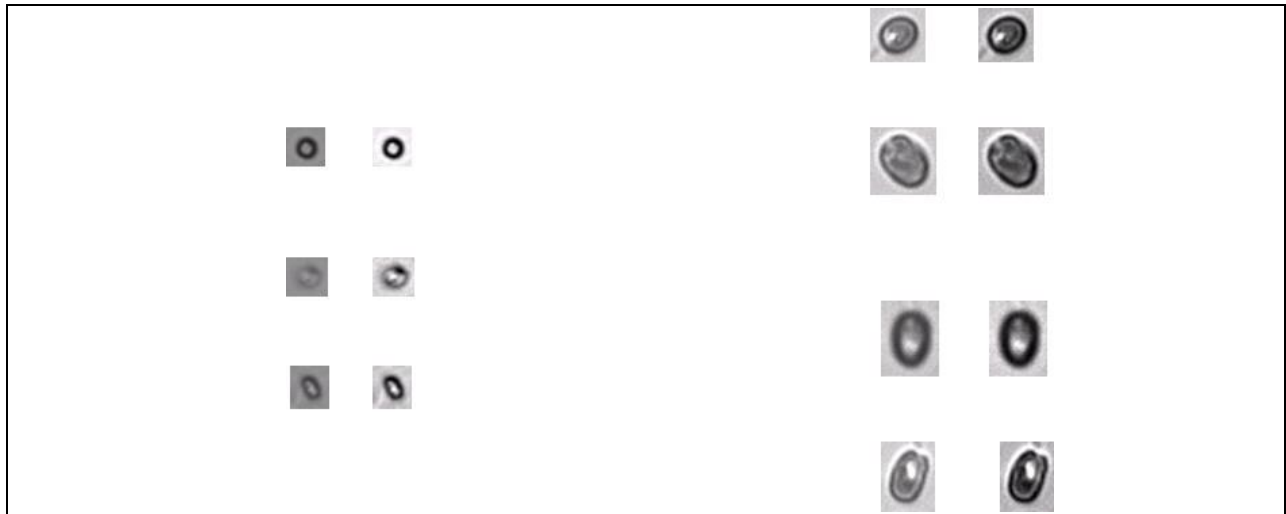
Figure 14. FlowCAM® Tetraselmis images - Analog camera images on left and digital camera images on right.
