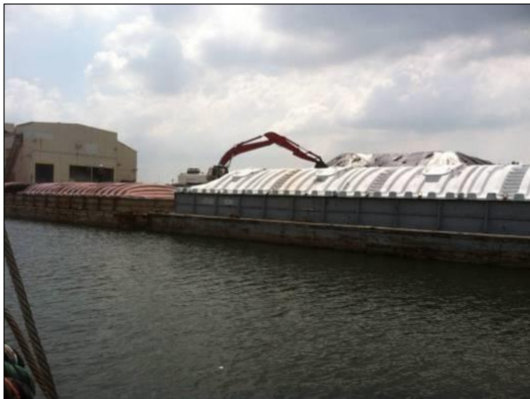
Figure D-2. Loaded barges rafted at construction materials site (upper). Covers being installed to protect cargo on hopper barge, note added height (lower).
