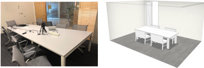
Fig. 5: We use an off-the-shelf app called MagicPlan to generate geometry proxy. Input: a real-world room (left); Output: the captured 3D model of the room (right) without high-level details, which is used by the runtime geometric acoustic simulator.
