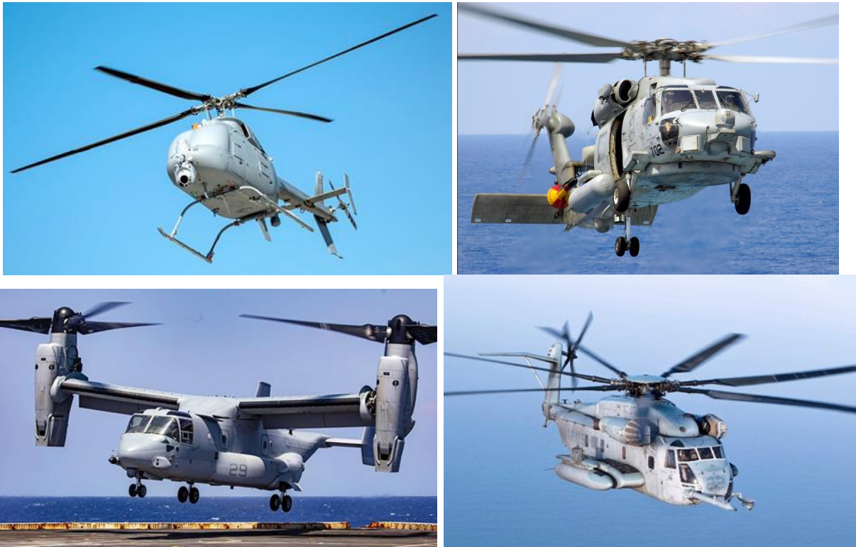
Figure 2: Aircraft used as the basis of rotor response analysis: (top left) MQ-8C Fire scout (Bell 407); (top right) Sikorsky SH-60; (bottom left) Bell/Boeing V-22, and (bottom right) Sikorsky CH-53E
