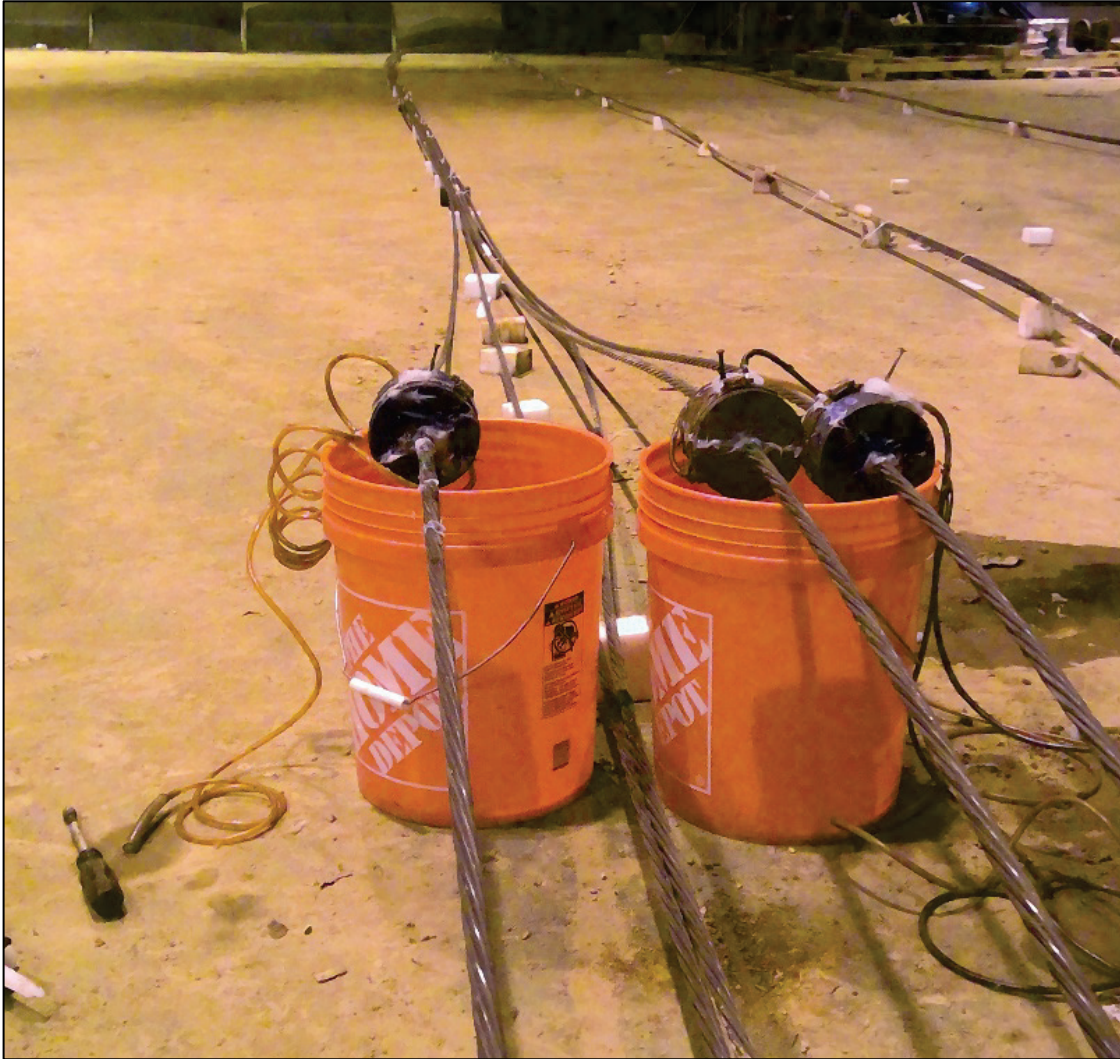
Figure 4. Multiplexed corrosion flow cells being used to corrode three separate seven-strand cables. Due to the portability of the cell, corrosion defects may be introduced at any point in the cable length without the need for large reactor beds.
