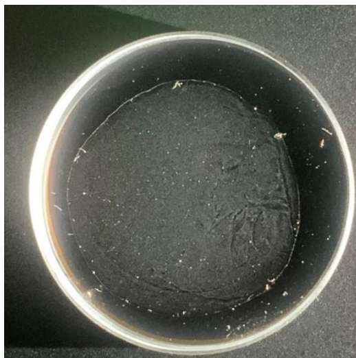
Figure 12: Fused silica substrate with optically thin Eu:BAM coating.
