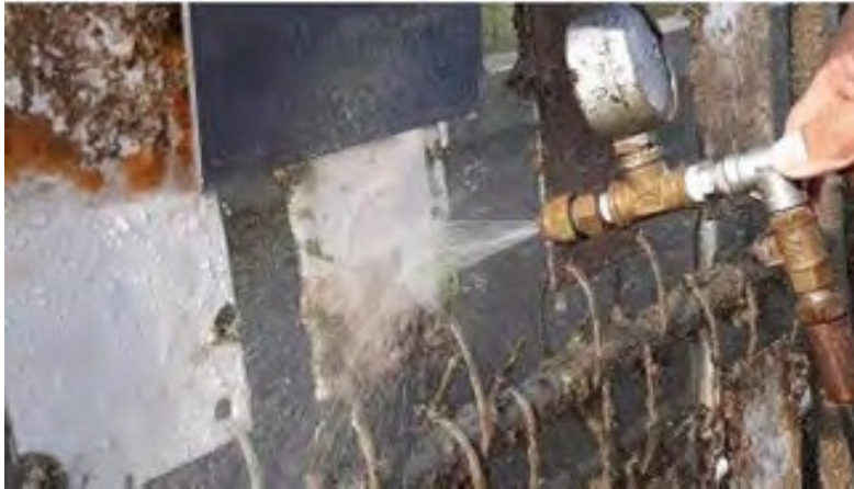
Fig. 5. Lower half of each coated panel was cleaned with (50 PSI) waterjet pressure from a pressure washer where desired pressure was achieved manually by valve control and nozzle gauge.
