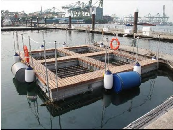
Fig. 1. Floating test platform located at a local marina for shallow submergence testing.
