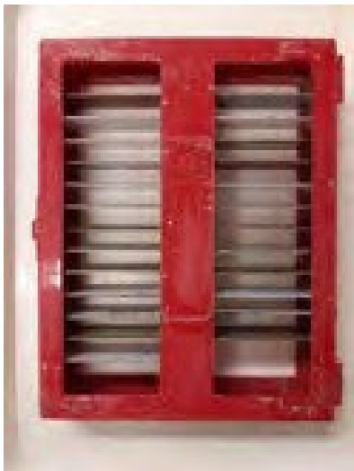
Fig. 7. Coated coupons on a cut-out microscope slide box to allow seawater flow-through.
