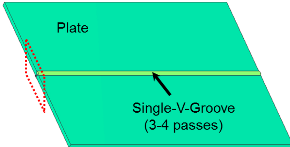
Figure 1. Representative CAD model showing the B2V.1 joint configuration. The red box (left side) shows the magnified cross-sectional view shown in Figure 2 .
