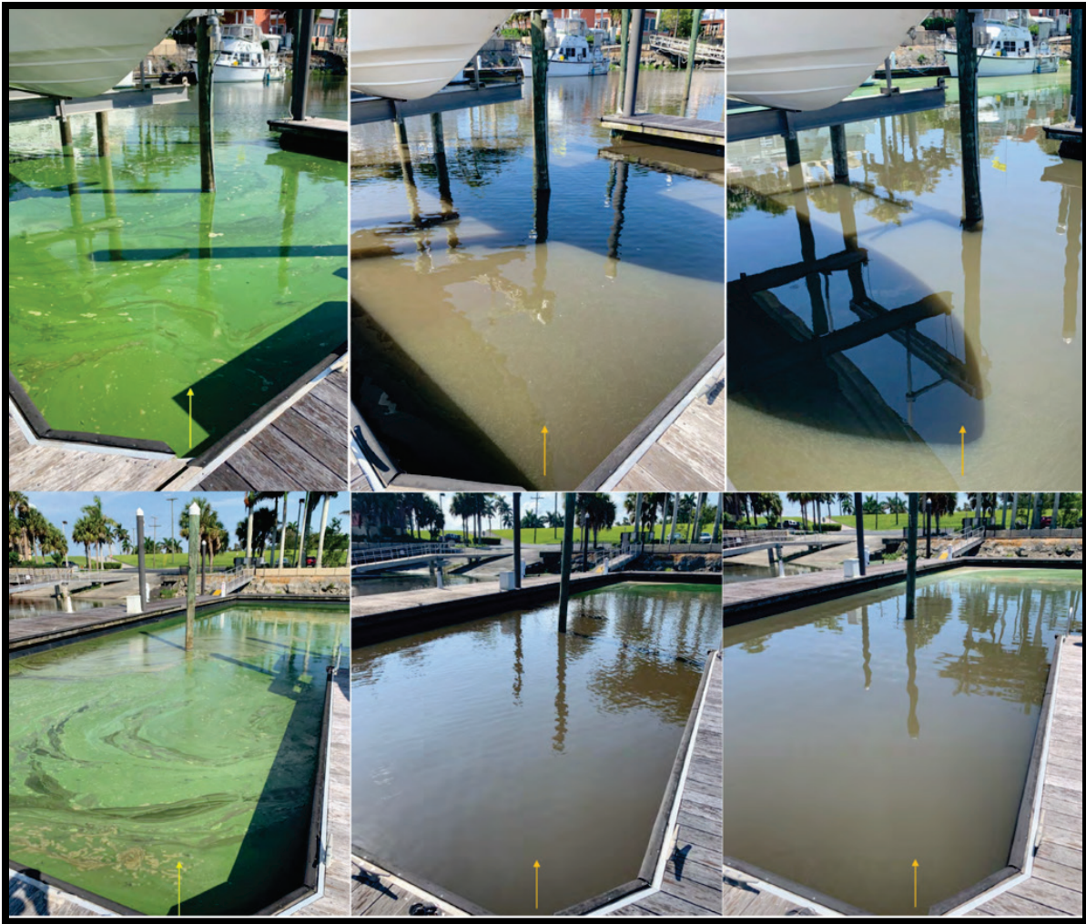
Figure 9. Time series of dock slips before, during, and after a peroxide-based algaecide treatment for CHAB control in a field demonstration on Lake Okeechobee, Florida, in July 2020.
