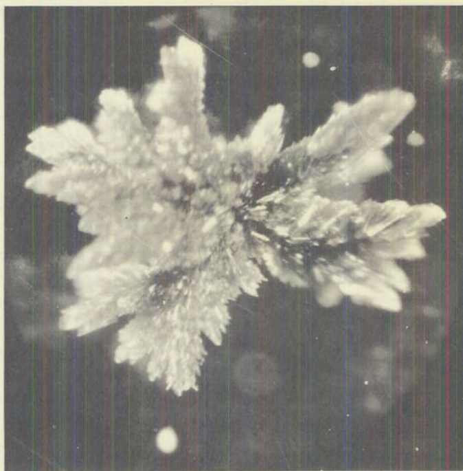
Figure 3 - Photomicrograph of \text{Fe}_3(\text{PO}_4)_2 \cdot 8\text{H}_2\text{O} crystals grown in gel medium
