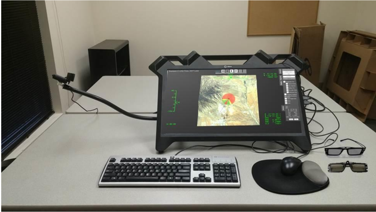
Figure 1. GUAVA desktop training device. The training device was developed to enhance the Soldier’s mental model of the 3D airspace in which they operate.
