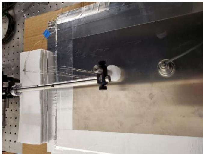
Figure 17. Splayed wire coupler receiving acoustic waves from the test piece and carrying them to a transducer.
