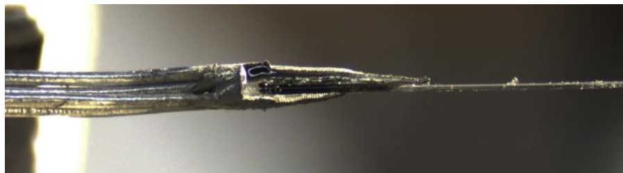
Figure 13. Silica fiber spliced to splayed aluminum acoustic coupler.
