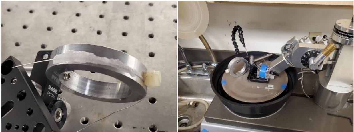
Figure 16. Polishing apparatus for tapering the aluminum wire.
