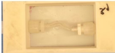
Figure 5: Static Bioreactors were designed to hold the engineered heart tubes in three different positions from different timepoints from the looping process.
