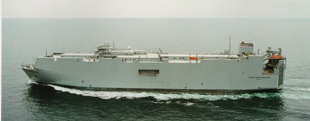
Figure 1. M/V Cape Washington (AKR-9961, MARAD photo) serves as the test facility for Navy BWMS testing. Ship displacement is 22,145 t.(light displacement), 53,500 t.(full load). Ship dimensions (in feet) are: length 697', beam 106', draft 38'. Ship speed is 14.7 kts. Image source: MARAD, posted on http://www.navsource.org/archives/09/54/549961.htm .
