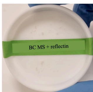
Figure 14: Incorporation of reflectin protein onto BC microspheres and casted on hydrophobic surface
