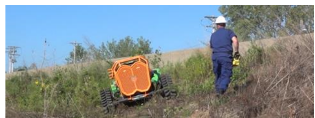
Figure 2. Green Climber LV600 with operator using a Bluetooth control belt-pack (yellow) to direct the LV600 movements. (Source: U.S. Coast Guard)
