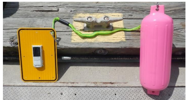
Figure 4. GlobalStar SmartOne Solar tracker on a mounting plate with high-visibility fender (Source: U.S. Coast Guard).
