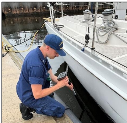
Figure 1. Testing of MarCum camera attached to telescoping rod (Source: U.S. Coast Guard).
