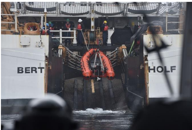
Figure 2. Recovery from the stern notch on USCGC BERTHOLF (Source: U.S. Coast Guard).
