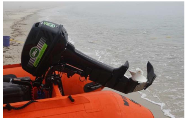
Figure 1. Elco 20 HP electric outboard during trials at the R&D Center (Source: U.S. Coast Guard).
