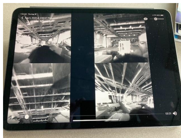
Figure 2. Remote Quad Screen Display from the ball cameras (Source: U.S. Coast Guard).
