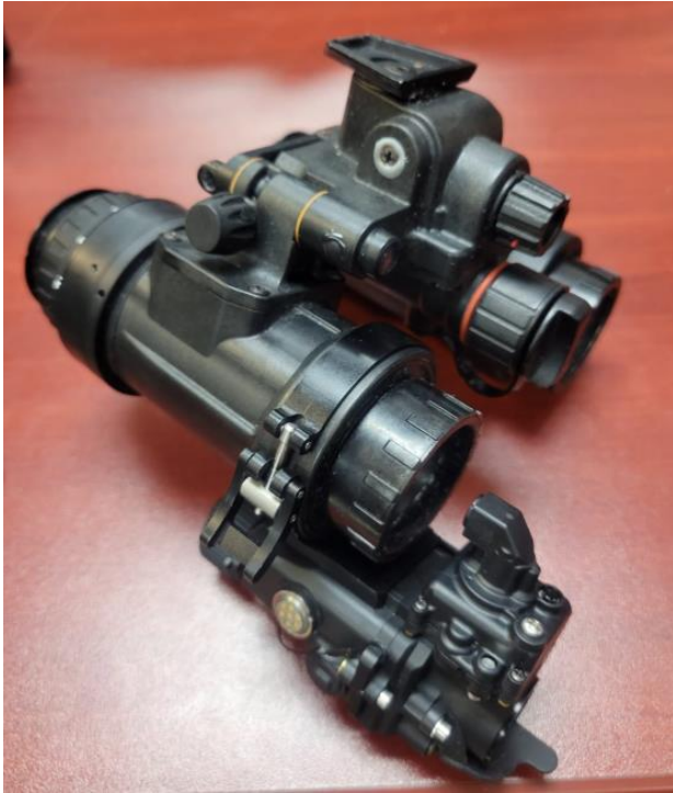
Figure 4. ECOTI installed on BNVD-1531 (Source: USCG).
