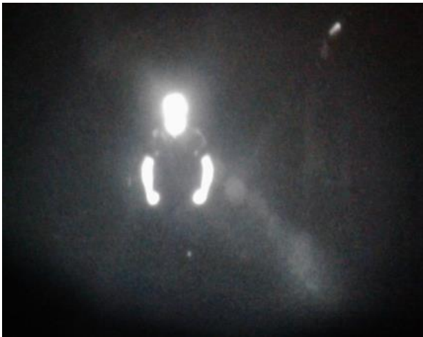
Figure 5. RDC personnel in RDC light lab. ECOTI is paired with GPNVGs. All lights in light lab are turned off to show clip-on utility in total darkness (Source: USCG).
