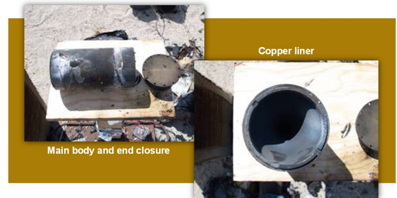
Slow Cook-off No damage to main body, end closure, or copper liner Heating rate was 3.3°C/hr
