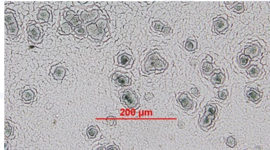
Microscope Images Reveal Basic Copper Carbonate Particles
