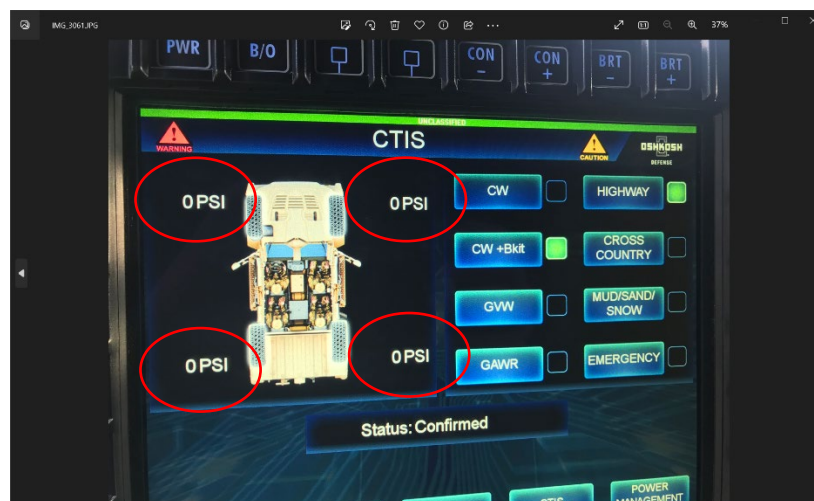
Figure 15 JLTV DSDU CTIS tire pressure targets (under threat)
