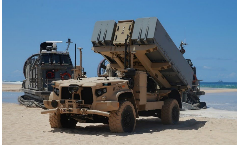
Figure 5 The semi-autonomous JLTV based NEMESIS SSM launcher system
