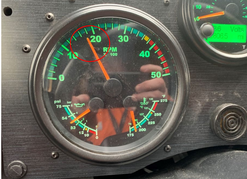
Figure 12 JLTV dashboard instrument showing engine speed (under threat)
