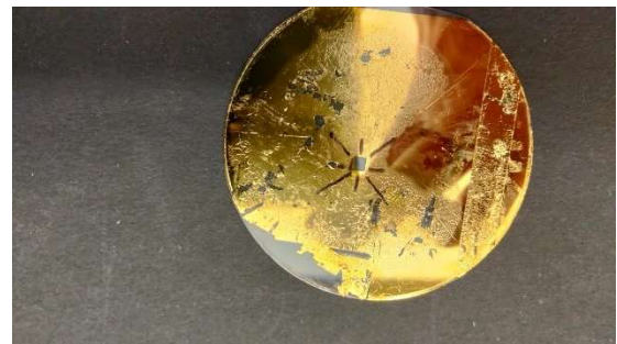
Fig. 31 Spin coated PCBM film on sapphire with a gold foil protecting layer. The EBL window based on the metal frame/lift off produced is also seen. This sample was subjected to UV-Vis before 8.5 hours of EBL and after EBL. No data could be recorded band gap before and after EBL for this PCBM film. The PCBM on EBL window is supposedly etched off due to acetone application in photoresist removal process.
