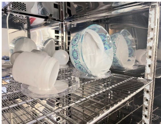
Figure 13. The mixing containers cured in the oven, allowing them to be cleaned easily.
