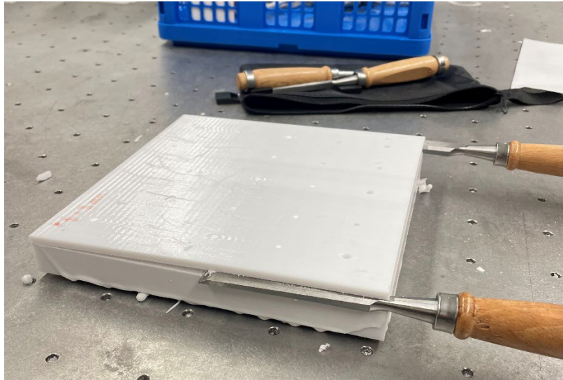
Figure 14. An example of using the chisels to remove the lid slowly.
