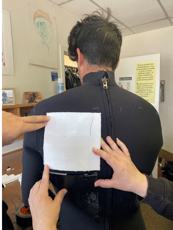
Figure 17. Preplacing the pieces on the suit for maximum coverage.
