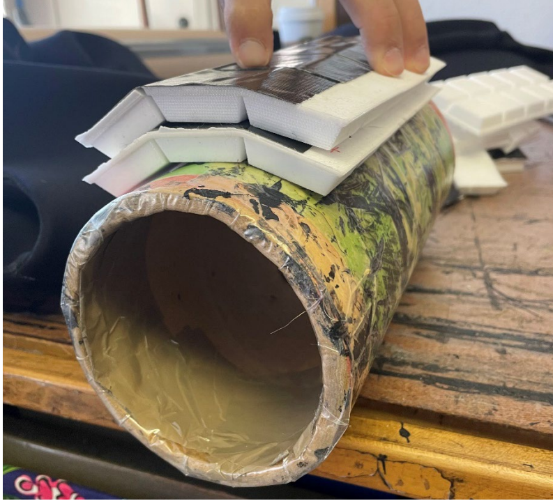
Figure 18. Pre-curving the pieces over the cardboard roll.
