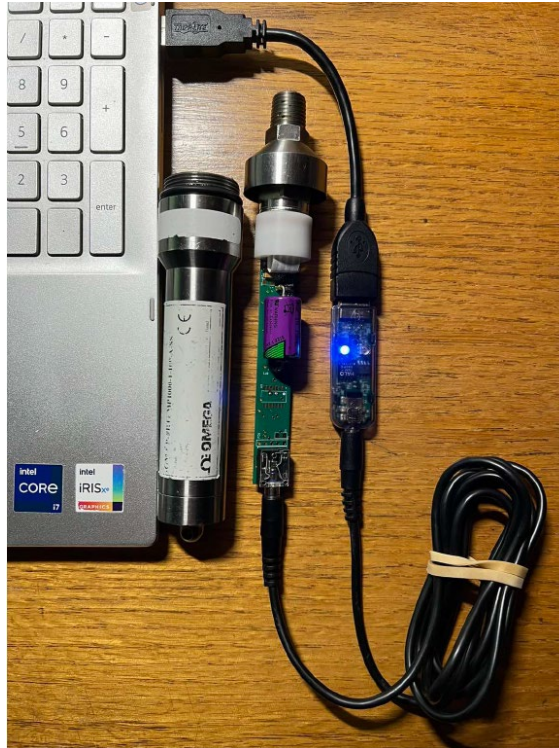
Figure 21. The Omega data logger connected to the computer. Source: [11].
