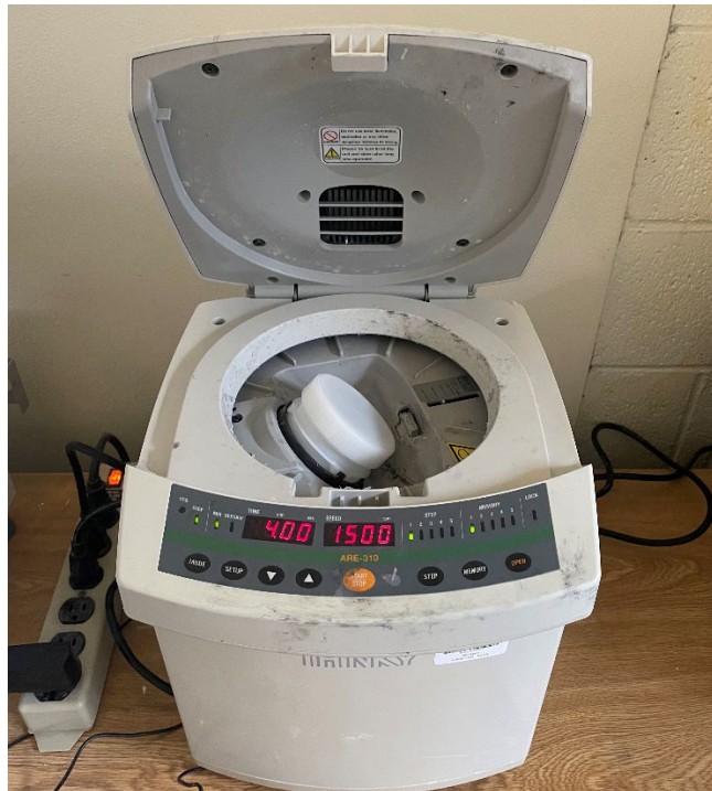
Figure 9. The planetary centrifuge prepped with the correct settings to start mixing.
