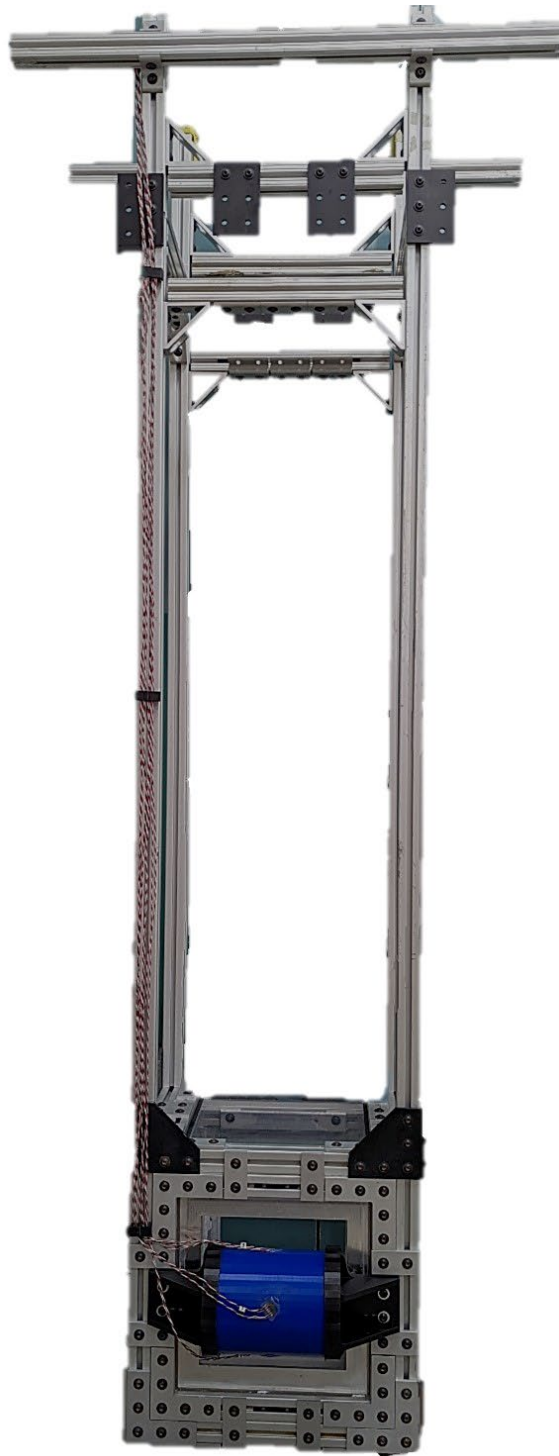
Figure 4. Composite Test Rig with PLA Cylinder Mounted
