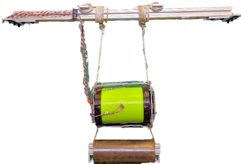
Figure 10. PLA Cylinder on Composite Test Rig with the Hold Bar
