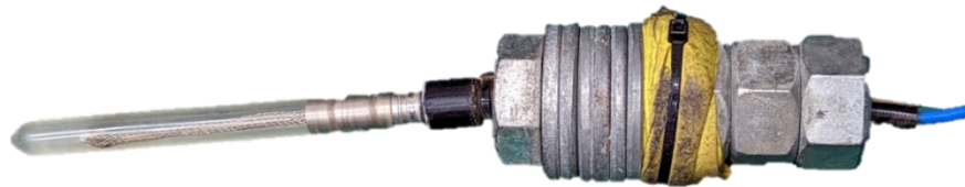
Figure 8. Tourmaline ICP Underwater Blast Sensors by PCB Piezotronics
