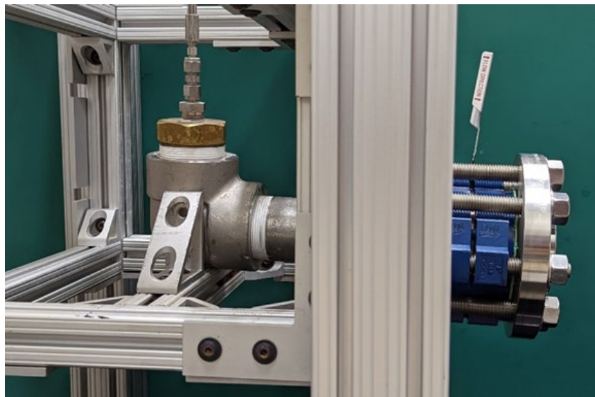
Figure 11. Rupture Disk Assembly on the Shock Test Rig
