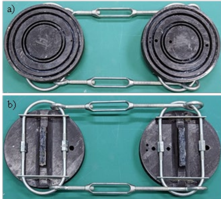
a) Inside view with grooves displayed. b) Outside view with U-bolts and turn buckles attached.
